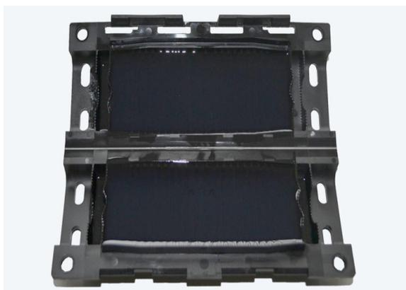
The gel-filled cable joint technique is a new system with special advantages. It is quick and easy to install and reduces the chance of assembly errors. The impact-resistant case is connected by a hinge for easy installation. After closing the cable joint the special gel flows together and ensures a good sealing and insulation of the connection. After installation, the cable joint can be put directly in use. No special tools required. Good adhesion to metals and plastics.
